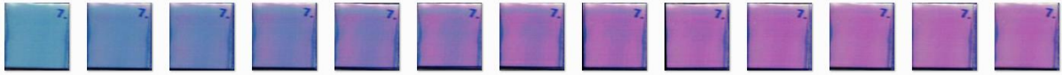
Figure 1. Typical set of digital images of a photocatalytic film on a sample of commercial self-cleaning glass
